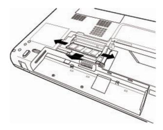
Figure 4-7 Removing the first memory
